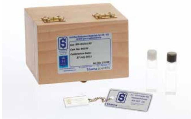
To allow users flexibility in use the reference is supplied with certified wavelength and absorbance values at two different bandwidths, 1.0 nm and 5.0 nm. Nominal values are given below.
