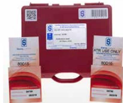
The alternative version has a film thickness of  $65 \mu\text{m}$  and also has certified peaks in the Near-Infrared, covering wavelengths from  $3000 \text{ cm}^{-1}$  to  $9.000 \text{ cm}^{-1}$  ( $3.3$  to  $1.1 \mu\text{m}$ ).
