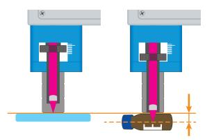
Adjustable focus position enables to vary the measurement position from the sample surface to the inside of the bottle.
