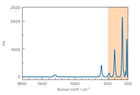
$\ensuremath{\mathsf{PR-1w}}$  allows to perform the low wavenumber measurement down to 200 cm  $^{-1}.$
