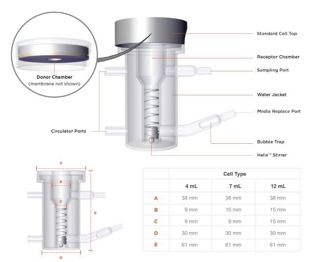
Hanson VDCs are available in the three standard sizes in amber or clear glass, and in custom sizes upon request. The 7 mL "Standard" VDC is recommended by the US FDA for topicals.
