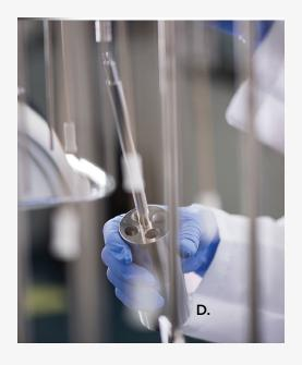
The Rotating Cylinder complies with USP <724> and holds patches up to  $5 \times 14$  cm in size (f.). For larger patches up to 10 x 14 cm in size, a Rotating Cylinder with Extension (d.) is available (both pieces are matched and must be purchased together). The Rotating Cylinder and Extension are serialized and come with a Certificate of Conformance.
