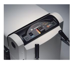
The easy-to-use controls on the Media-Mate panel allow one push to initiate a complete media measurement, deaeration, and dispense cycle, filling all 6 or 7 dissolution vessels in less than 5 minutes.
