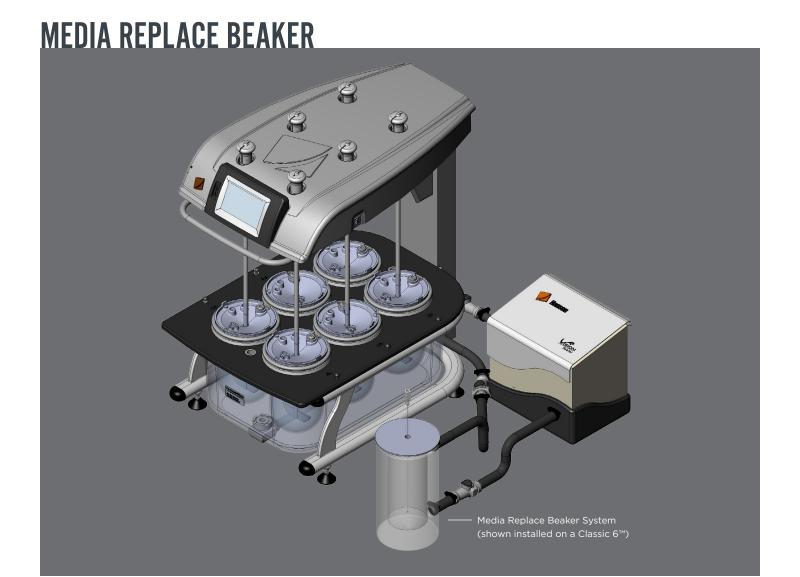
The Media Replace Beaker system is an optional accessory available for a new or existing Classic 6 dissolution tester. It allows the Classic 6 to simultaneously warm an additional one liter of media while performing a six-sample dissolution test. The warmed media can then be replaced either manually into the dissolution vessels or automatically using the Vision AutoPlus autosampler.
