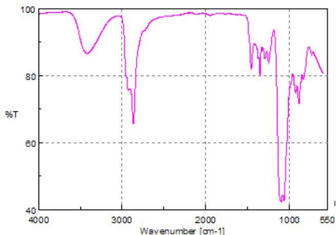
**Figure 6.** Spectrum of brake fluid.
