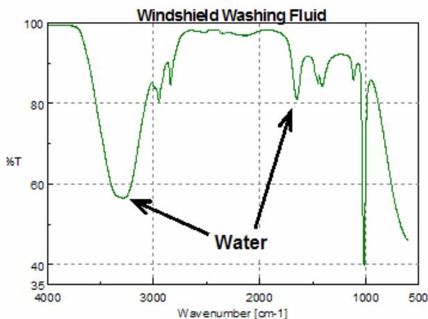
**Figure 2.** Spectrum of windshield washing solution. Infrared analysis using Attenuated Total Reflectance (ATR) accessories like the diamond single-reflection micro-ATR
