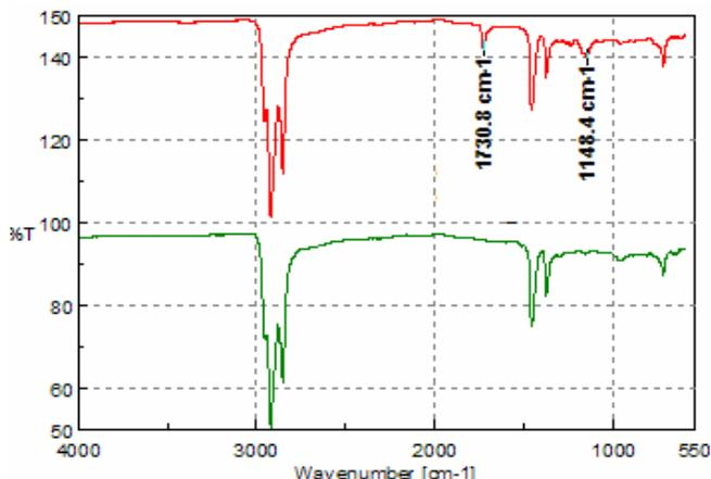
**Figure 5.** Analysis of 10W30 engine oil (green), power steering fluid and two transmission fluids (red)
