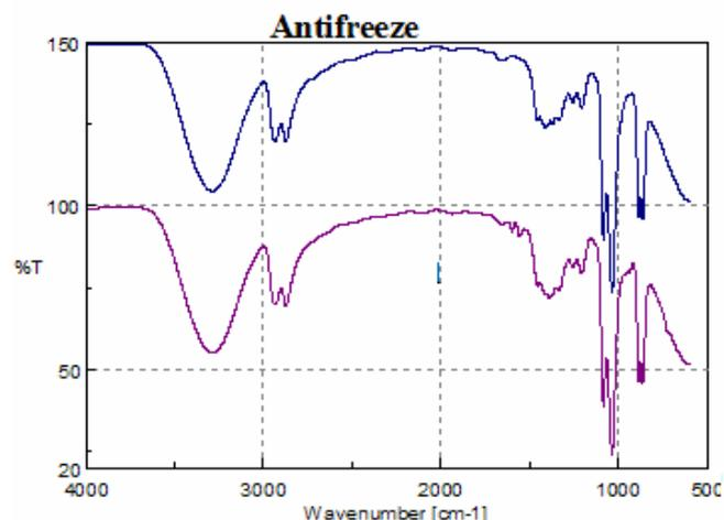
**Figure 3.** Spectra of two samples of anti-freeze, normal-blue and the extended lifetime-purple.
