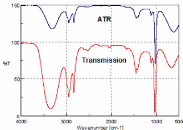
**Figure 1.** Transmission and ATR spectra of methanol.
