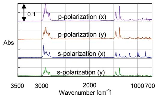
Figure 3: Spectra of a PP film measured by polarized ATR
