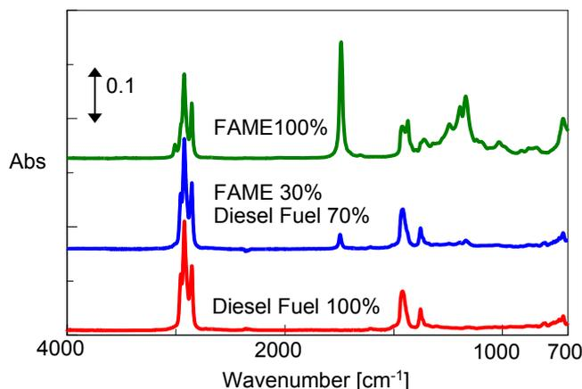
Fig. 2. IR spectra of FAME and diesel oil
