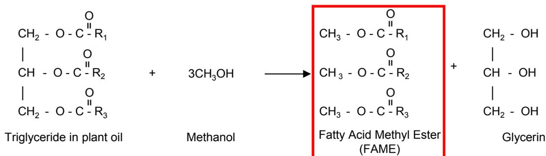
Fig. 1: Reaction pathway from vegetable oil to FAME
