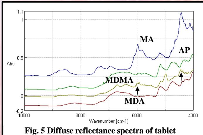
Fig. 5 Diffuse reflectance spectra of tablet
