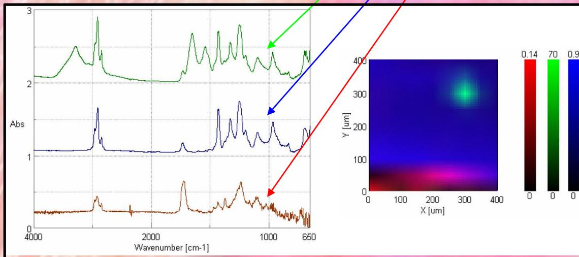
By analyzing the spectra in Fig. 3, it was confirmed that multi-layer film roughly consisted of two components, PVA (red), PVC (blue), and protein (green) was existing in the multi-layer film. By showing color distribution map utilizing specific peaks for each component on the RGB display (Fig. 4), components distribution became clear, enabling to detect the impurity which could not be identified by observation image.
