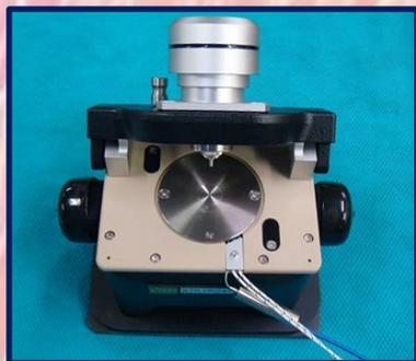
**Fig. 2 ATR Heating Single Reflection ATR accessory**
