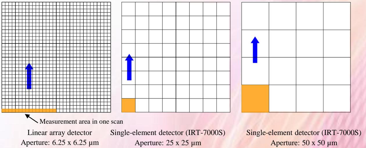
**Fig. 1 Comparison of measurement area in 200 x 200 μm area**
