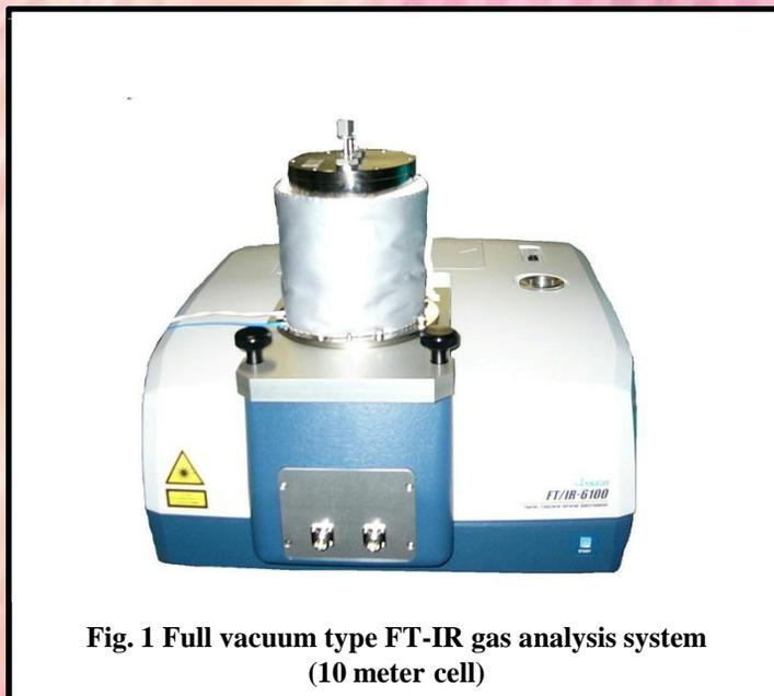
**Fig. 1 Full vacuum type FT-IR gas analysis system
