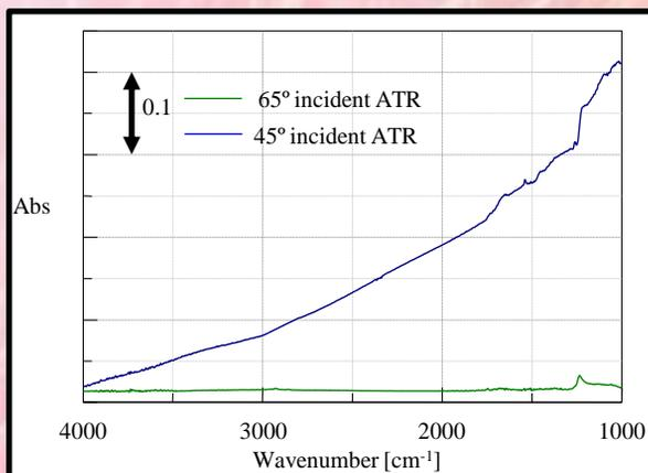
Fig. 2 Oxide Film Spectrum on Si Wafer
