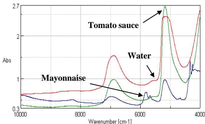
**Fig. 4 Measurement example using laboratory dish**
