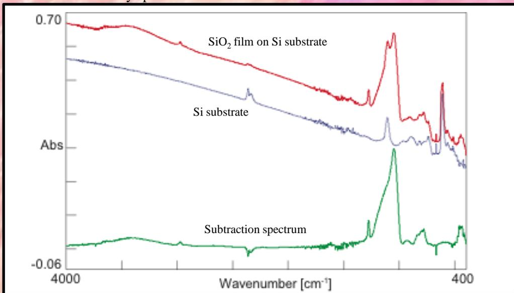
Fig. 1 Transmission spectrum of SiO<sub>2</sub> film under 0° incident angle condition
