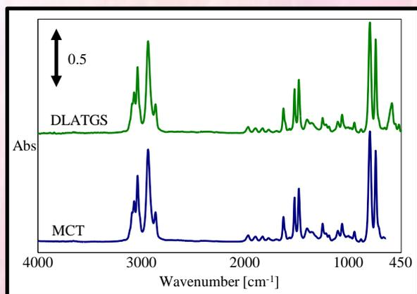
**Fig. 1 Spectrum of a polystyrene film using the new DLATGS and an MCT detector**
