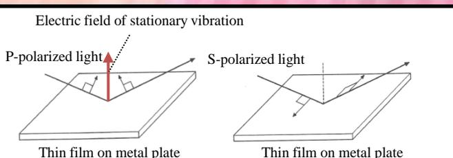
Fig. 1 Diagram of IRRAS method
