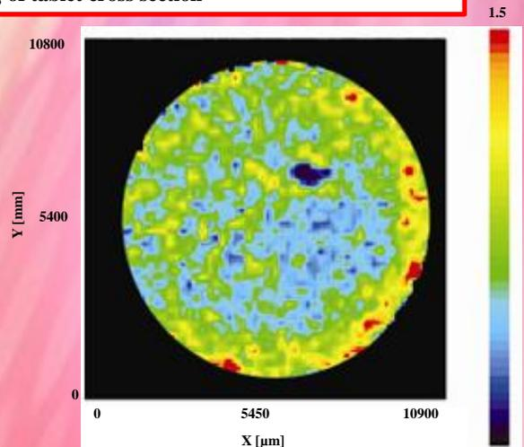
Fig. 6 Imaging of surface layer Peak ratio :  $4380 \text{ cm}^{-1}/4680 \text{ cm}^{-1}$
