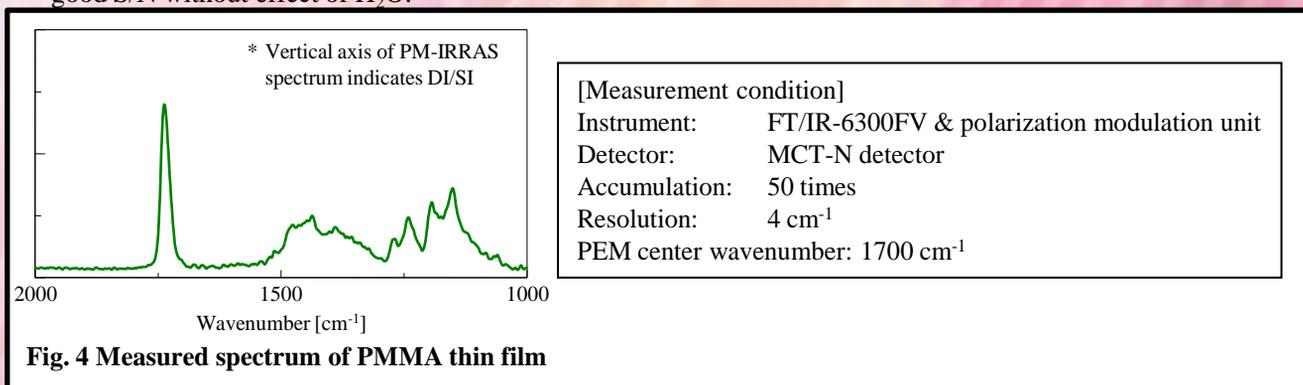
**Fig. 4 Measured spectrum of PMMA thin film**
