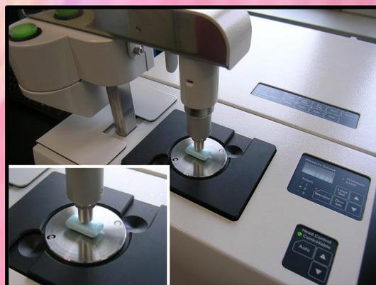
Fig. 1 Granular gum place on ATR crystal
