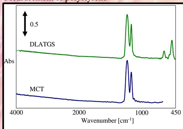
**Fig. 2 Spectrum of a Teflon sheet with using the new DLATGS and an MCT detector**
