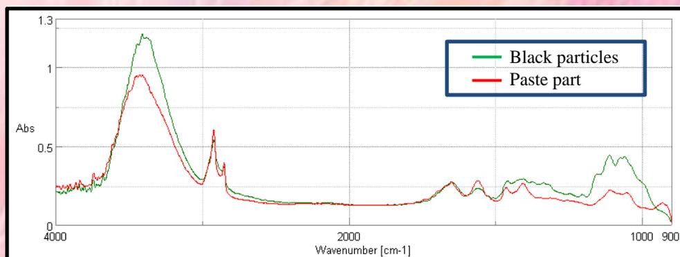
Fig. 3 Spectra of the paste part and black particles (After ATR correction)
