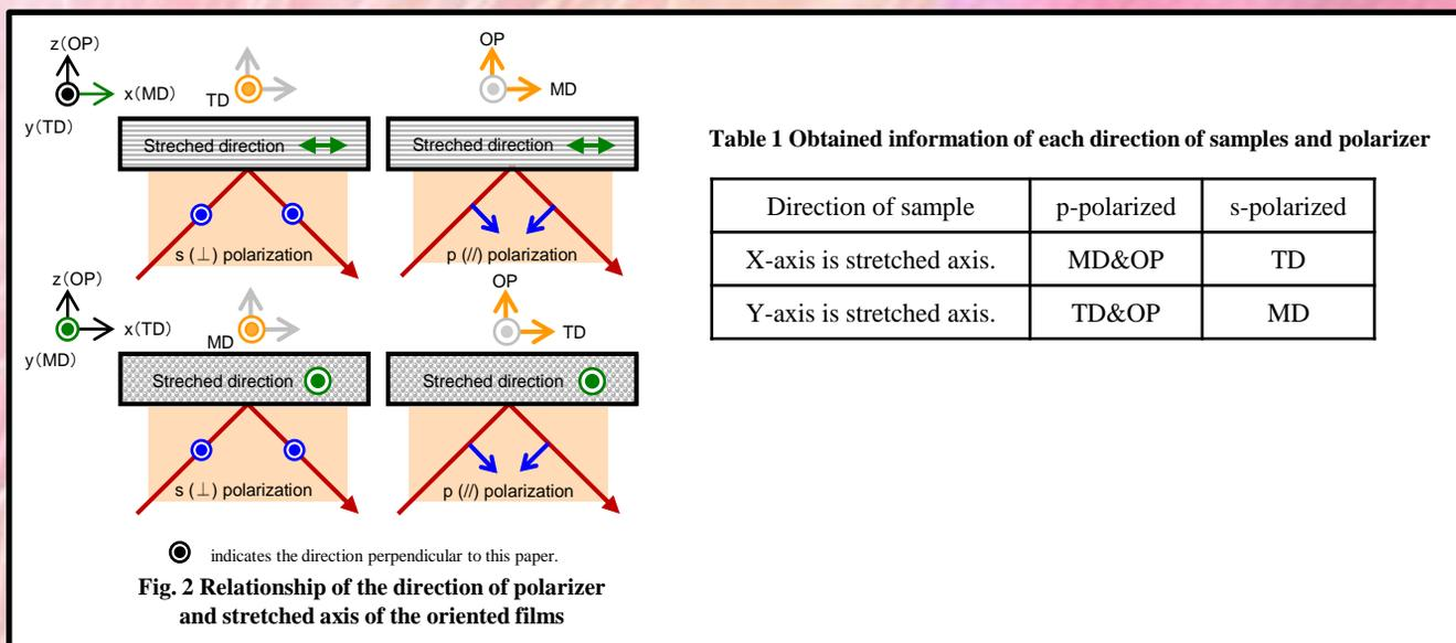
**Table 1 Obtained information of each direction of samples and polarizer**
