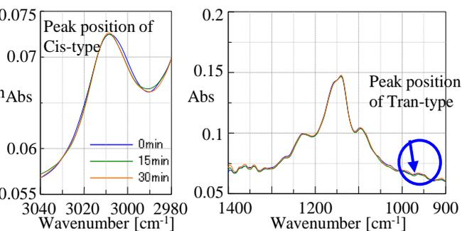
Fig. 4 Spectra under N<sub>2</sub> purged condition
