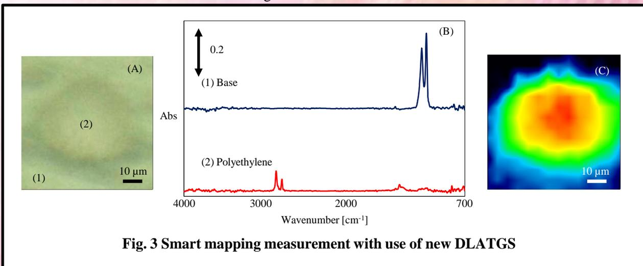
**Fig. 3 Smart mapping measurement with use of new DLATGS**
