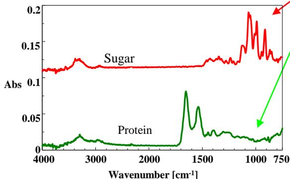
The powder sample that can't be identified by visible observation was observed by using of the fluorescence observation accessory and it's IR spectrum was measured at both green color area which observed as fluorescence and black color area.
