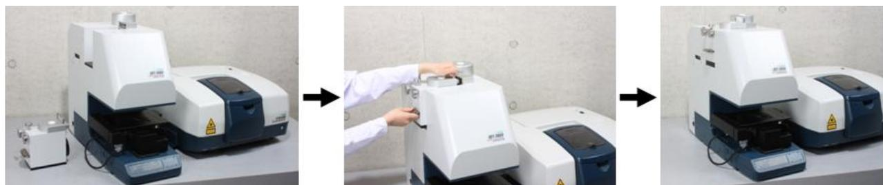
**Fig. 1 Detector replacement by using detachable detector unit**
