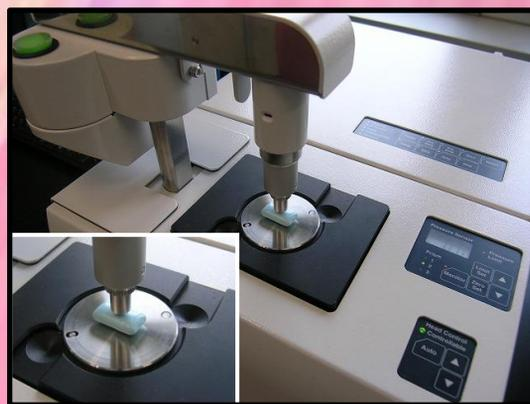
Fig. 1 Granular gum place on ATR crystal
