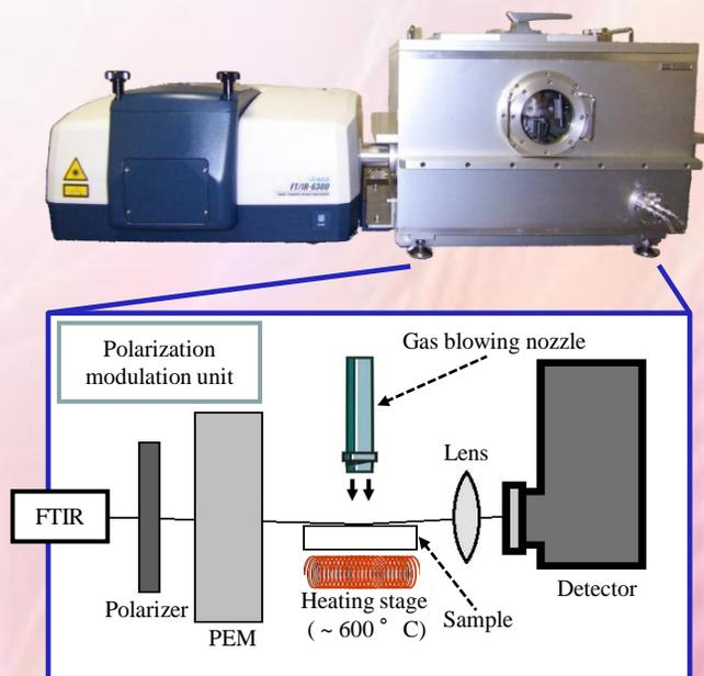
**Fig. 3 Appearance of FT/IR-6300FV & Polarization modulation unit (upper)
