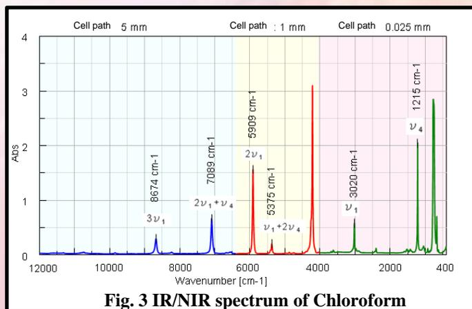
**Fig. 3 IR/NIR spectrum of Chloroform**
