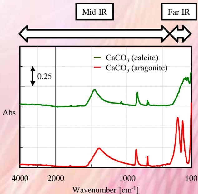
Fig. 3 Spectra of calcium carbonates that have different crystal structures (X-axis: 4:1 display, Y-axis: Offset)
