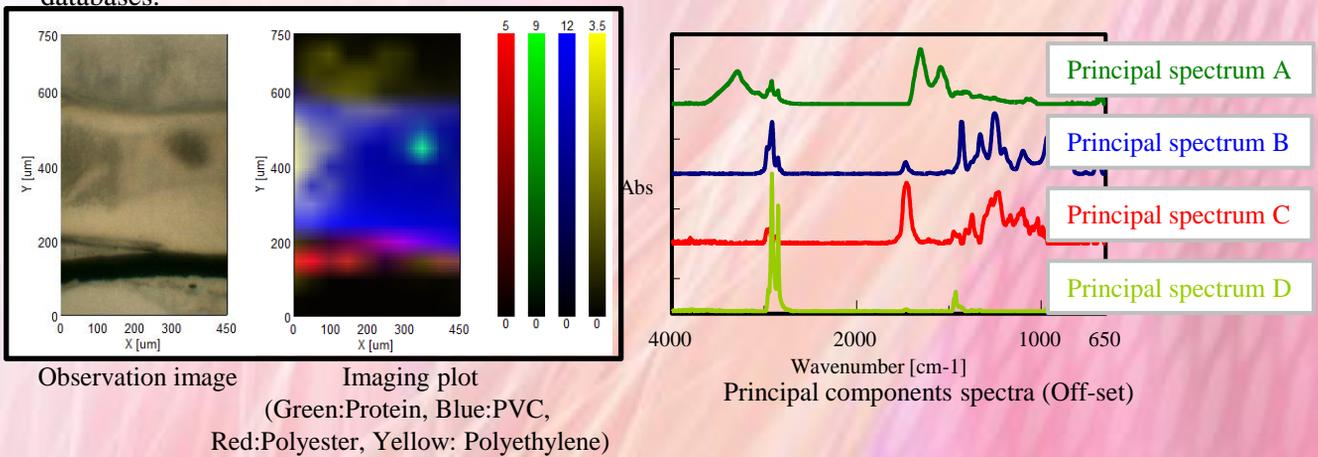
**Fig. 3** Imaging analysis result of multilayer film with “Model analysis”
