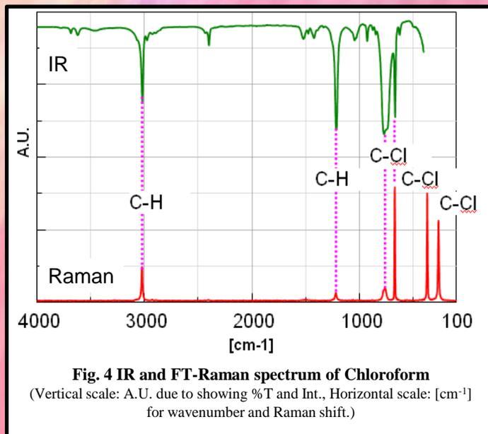
**Fig. 4 IR and FT-Raman spectrum of Chloroform**
