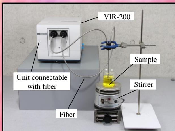
Fig. 1 VIR-200 + Fiber connection unit
