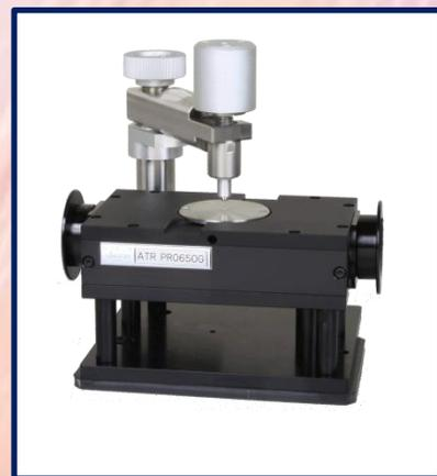
**Fig. 1 Single Reflection 65° Incident ATR
