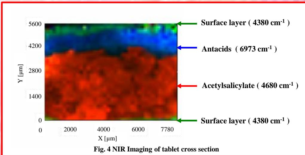
Fig. 4 NIR Imaging of tablet cross section
