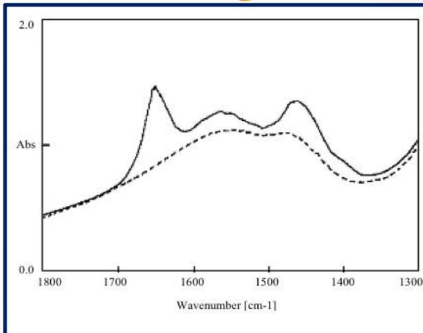
**Fig. 1 Overlaid spectra of 2% myoglobin in Heavy water, and Heavy water**
