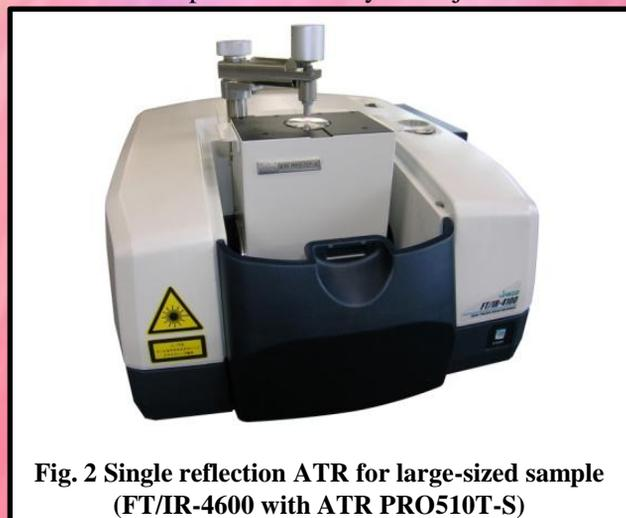
**Fig. 2 Single reflection ATR for large-sized sample (FT/IR-4600 with ATR PRO510T-S)**
