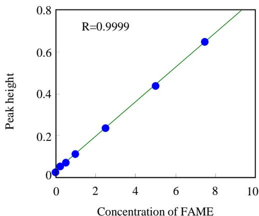
**Fig. 5 EN calibration curve of FAME**
