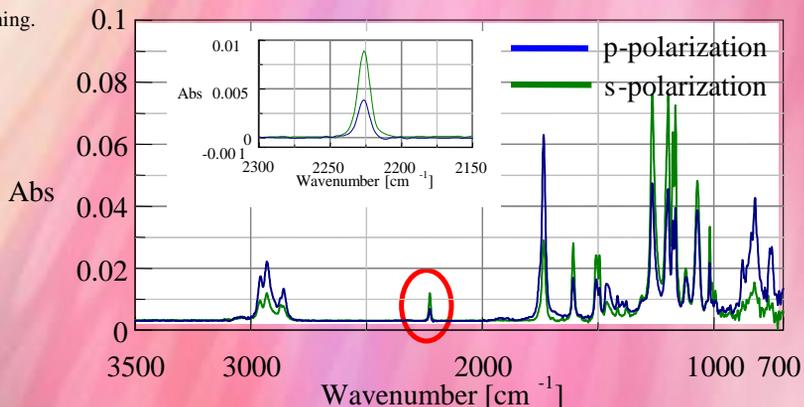
**Fig. 5 Spectra of a TN crystal measured by polarized ATR**
