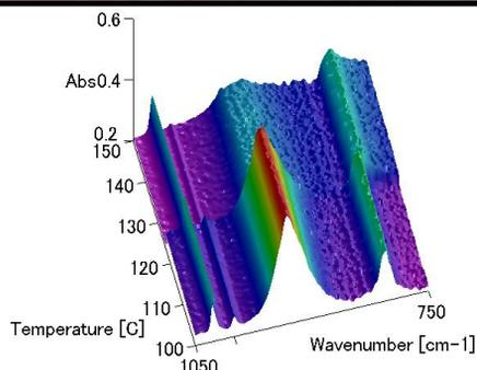
Fig. 2 3D spectrum of benzoic acid
