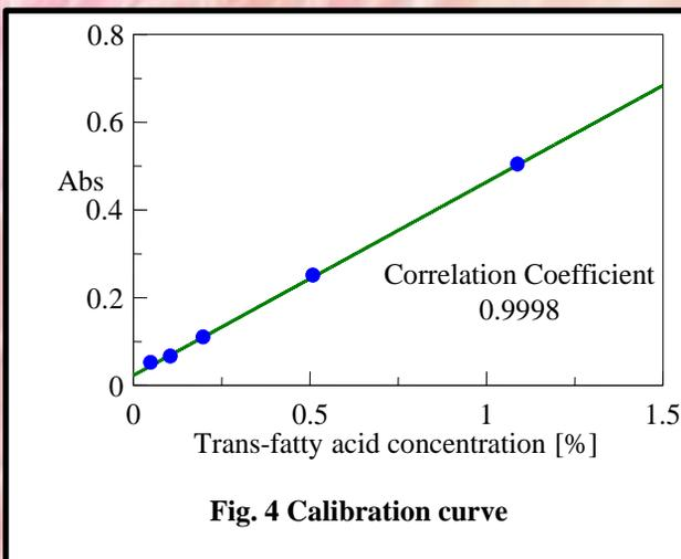
Fig. 4 Calibration curve
