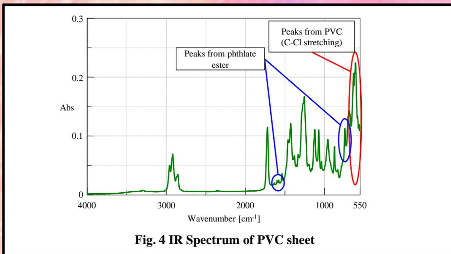
Fig. 4 IR Spectrum of PVC sheet
