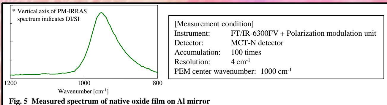
**Fig. 5 Measured spectrum of native oxide film on Al mirror**
