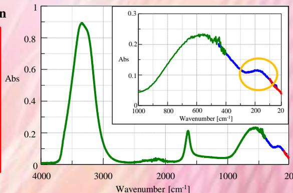
**Fig. 2 ATR spectra of pure water (Upper right: Enlargement below  $1000\text{ cm}^{-1}$ )**
