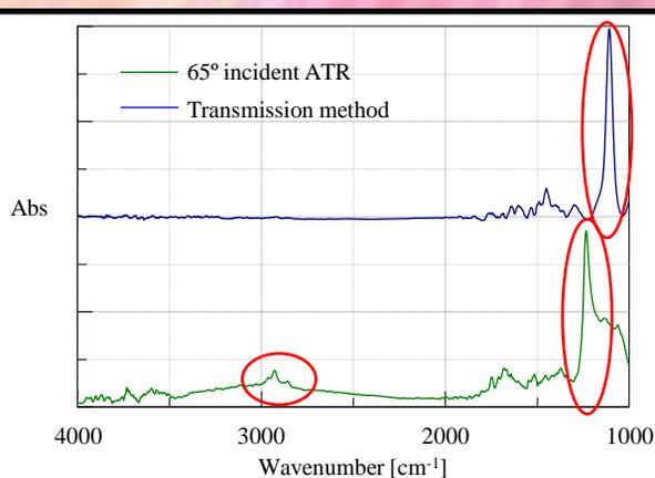
Fig. 3 Oxide Film Spectra on Si Wafer
