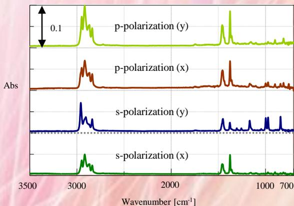
**Fig. 3 Spectra of a PP film measured by polarized ATR**
