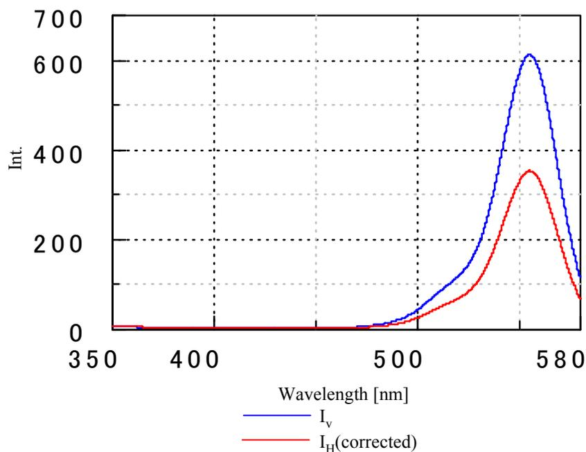
Fig. 1 Ex spectra of I<sub>V</sub> and I<sub>H</sub>(corrected)
