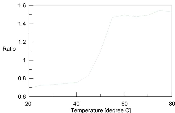
Fig. 4 Temperature control plot of fluorescence intensity ratio (332 nm/355 nm)
