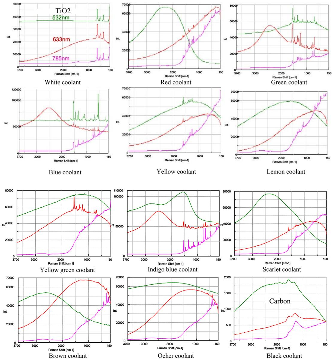
Fig1. Spectra data of colorant samples
