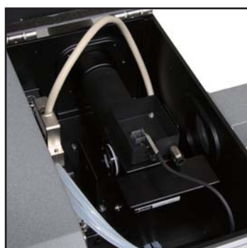
PTC-517 Peltier cell holder with emission optical unit and PML-534 high sensitivity FDCD detector
