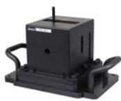
PM-491 Permanent Magnet, 1.6 Tesla
